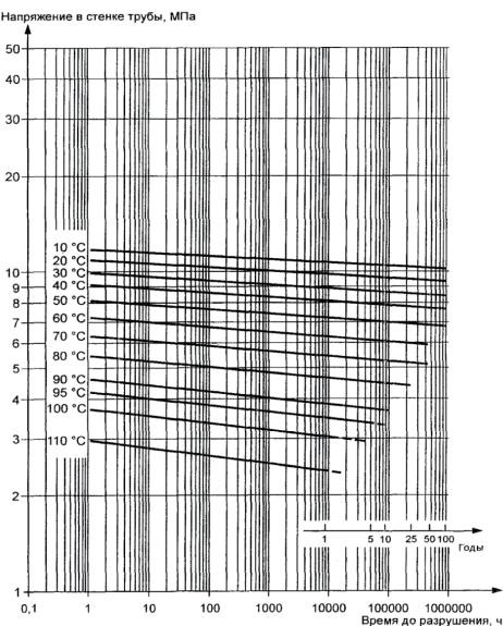
$$\lg(t) = -219 - (62600,752/T) \lg(\sigma) + 90635,353/T + 126,387 \lg(\sigma)$$
